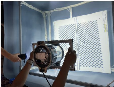
**Figure 3: Camera performing underwater targetless calibration over an open tank of freshwater**
